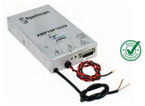
The XMPG is a modular 10kV @ 10W X-Ray generator designed to drive a grounded filament X-Ray tube via closed loop filamentary control of the 0 to 1mA emission current. The grounded filament supply is rated at 0-5 amps @ 3Vdc. The filament supply features an internally adjustable 0.5 to 2.5 amp filament preheat and a internally adjustable 0 to 5 amp filament limit.
