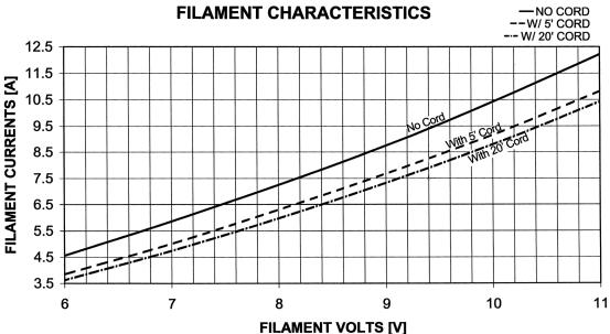
FILAMENT CORD: AWG #14, 2-CONDUCTOR
