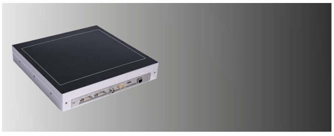
The 2824HS is a dynamic X-ray detector designed for industrial NDT, pre-clinical and clinical applications, with a pixel pitch of  $100 \mu m$  and a choice of high-efficiency, high-resolution Csl or Gadox scintillator. It is ideal for CBCT or fluoroscopy.
