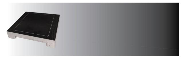
The 2121HS is a dynamic X-ray detector designed for industrial NDT, pre-clinical and clinical applications, with a pixel pitch of 100 µm and a choice of high-efficiency CsI or Gadox scintillator. It is ideal for CBCT or fluoroscopy.
