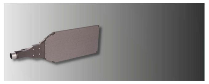
The 1510HS is a dynamic X-ray detector designed for industrial NDT applications, with a pixel pitch of 100  $\mu$ m and a Gadox scintillator. It is ideal for portable applications and weld inspection. The USB 3 interface handles data output, control and power supply. A handle can be attached for manual operation. Automatic exposure control (AED) allows the detector to be used with a portable source without synchronisation.
