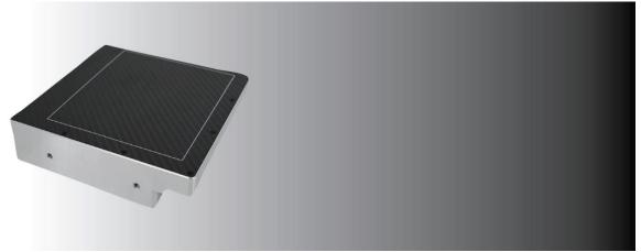
The 1412HR is a dynamic X-ray detector designed for electronics inspection, industrial NDT, pre-clinical and clinical applications, with a pixel pitch of 50  $\mu$ m and a choice of high-efficiency CsI or Gadox scintillator. It is ideal for CBCT or fluoroscopy.
