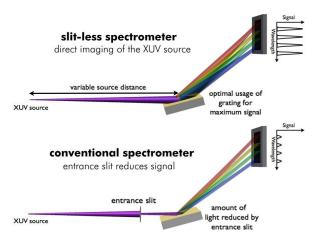
In practice, this allows for the collection of 15 to 25 times as much light from point-like radiation sources compared to a conventional spectrometer with a  $100\mu m$  entrance slit without degradation in spectral resolution. Typically, the signal-to-noise figure is improved by the same ratio. In some XUV/VUV experiments, this improved signal strength is the crucial step for realizing a measurement at all.
