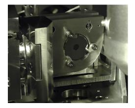
Double-mirror delay assembly XUV/VIS-IR for collinear beam refocusing. Temporal resolution of  $\pm 3as$ . 5 degrees of freedom. Spectral isolation of the cut-off region. Low wavefront distortion due to optically precise shaped segments
