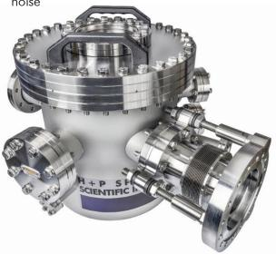
Compact spectrometer for in-situ HHG source characterization in the water window. Direct imaging of the source without entrance slit for maximum efficiency and day-to-day robustness. Undistorted beam in bypass mode. UHV vacuum setup. Longitudinal dimension <0.5m. All settings controlled remotely by software.
