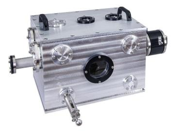
Turn-key system for investigation of high-order harmonic generation in laser-produced plasmas. Flexible motorized target setup for rotating and flat solid targets and gas targets. Multiple beam access options for two-color pumping of plasma. Integrated frequency-doubling stage. Spectral filtering stage for high-intensity beams.
