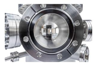
Beam-like view into in-line spectrometer. Reliable switching between bypass and spectroscopy modes by closed-loop positioners.
