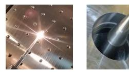
(1) Cross-drilled gas target allowing for long-term stable operation with constant gas flow. Convenient alignment with full beam due to high durability.
